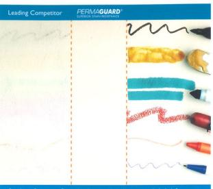
Results at 5 minutes: Cleaned with cotton cloth then isopropyl alcohol if necessary
